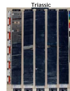
Fig. 4. Upper Triassic marine shales of the Fruholmen Formation from well 7214/3-1. The source rock interval has TOC 11.4 to 15.7 wt%.
