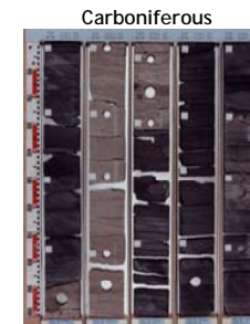
Fig. 6. Lower Carboniferous coals, mudstones and sandstones of the Soldogg Formation from well 7128/6-1. The coals have TOC 34 to 80 wt%, the mudstones have TOC 1.5 to 4.8 wt%.
