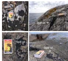
Fig. 4. Three different occurrences of heavily degraded spill oil along the south coast of Norway. Note matchbox for scale.
